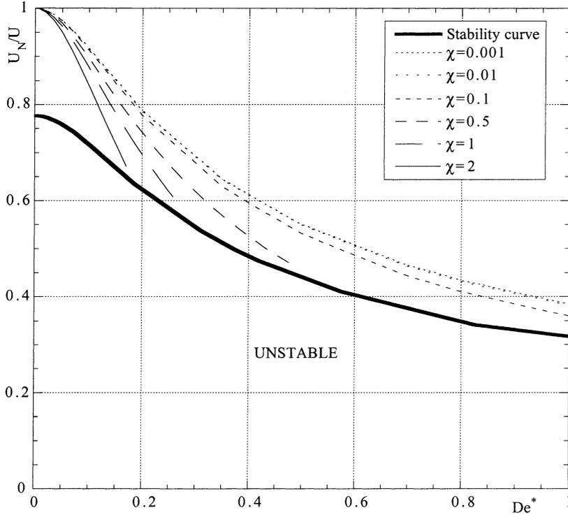
Fig. 4. Stability map of the PTT model fluid and ratio of Newtonian and PTT bulk velocities as a function of  $De^*$  and  $\chi$  for channel flow.
