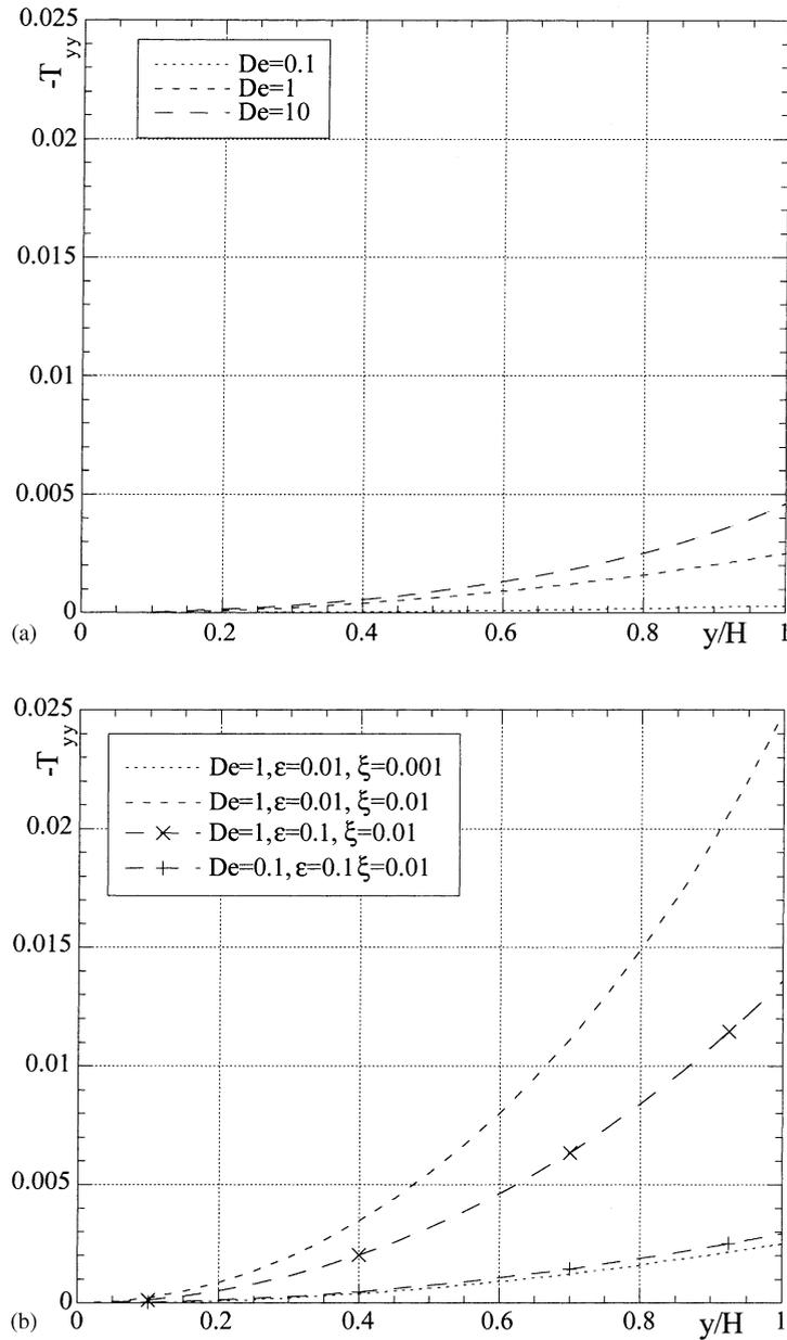
Fig. 9. Transverse profiles of cross-stream normal stress for channel flow. (a) Effect of Deborah number ( $\varepsilon = 0.01$ ,  $\xi = 0.001$ ); (b) effect of  $\varepsilon$  and  $\xi$ .
