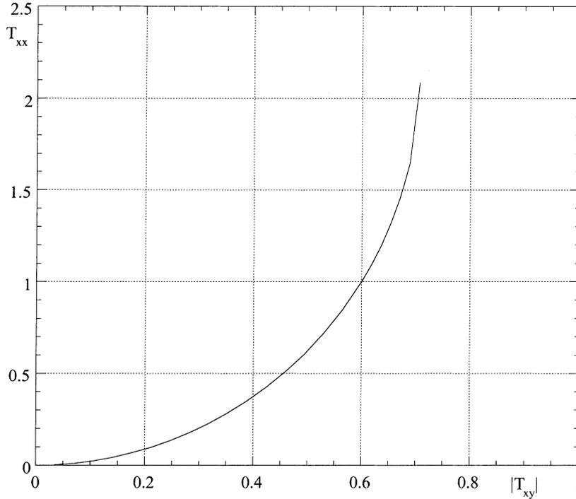
Fig. 11. Variation of the normal stress with shear stress across the channel for a situation just below critical ( $\xi = 0.2$ ,  $\varepsilon = 0.1$ ,  $De = 0.393$ ).
