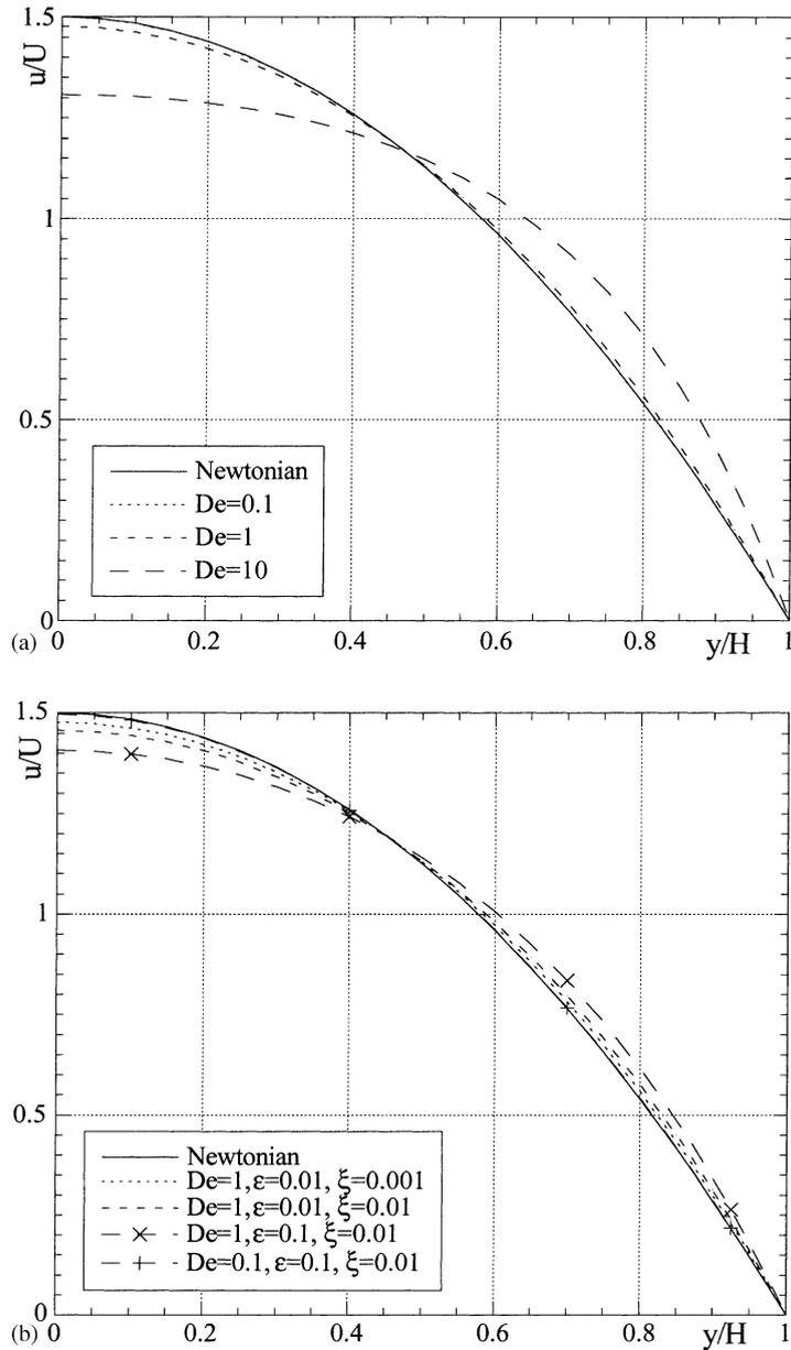
Fig. 6. Transverse profiles of axial velocity for channel flow. (a) Effect of Deborah number ( $\epsilon = 0.01$ ,  $\xi = 0.001$ ); (b) effect of  $\epsilon$  and  $\xi$ .
