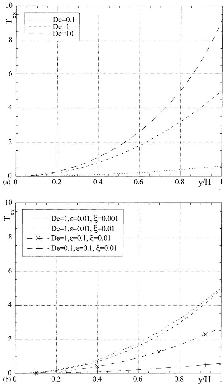
Fig. 8. Transverse profiles of streamwise normal stress for channel flow. (a) Effect of Deborah number ( $\epsilon = 0.01$ ,  $\xi = 0.001$ ); (b) effect of  $\epsilon$  and  $\xi$ .
