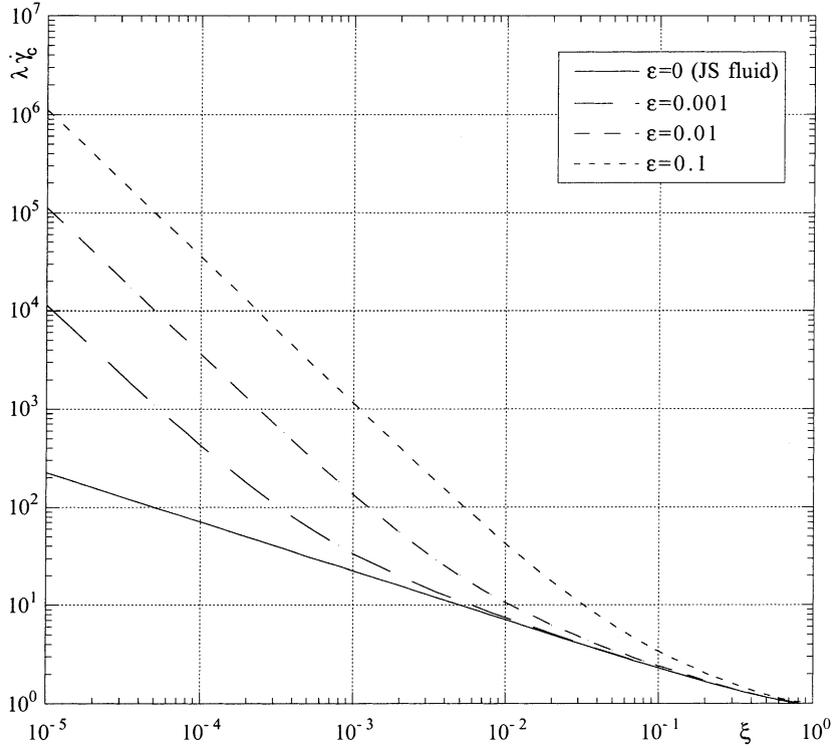
Fig. 3. Variation of the critical shear rate with the material parameters  $\epsilon$  and  $\xi$ .
