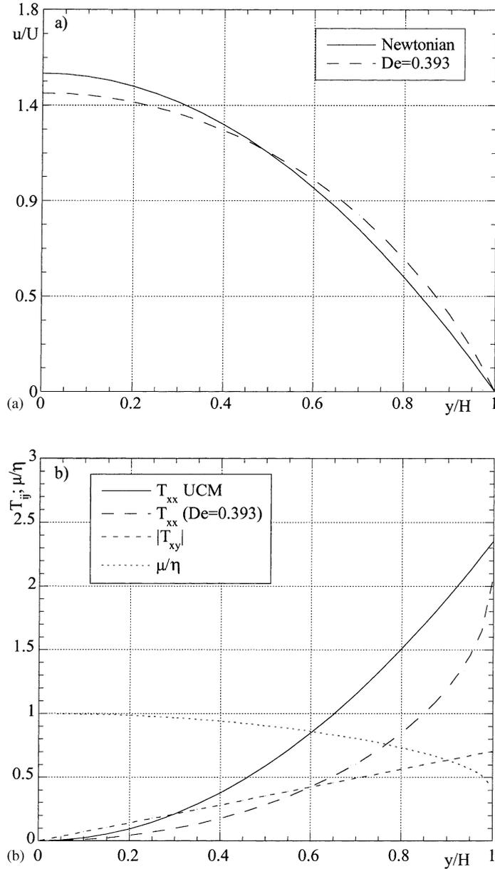
Fig. 10. Transverse profiles in channel flow for conditions just below critical at  $De = 0.393$  with  $\xi = 0.2$  and  $\varepsilon = 0.1$ : (a) velocity; (b) stresses and viscosity.
