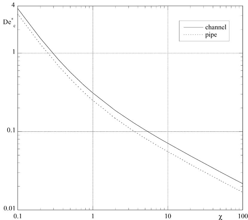
Fig. 5. Variation of the modified critical Deborah number with parameter  $\chi$  for channel and pipe flows.
