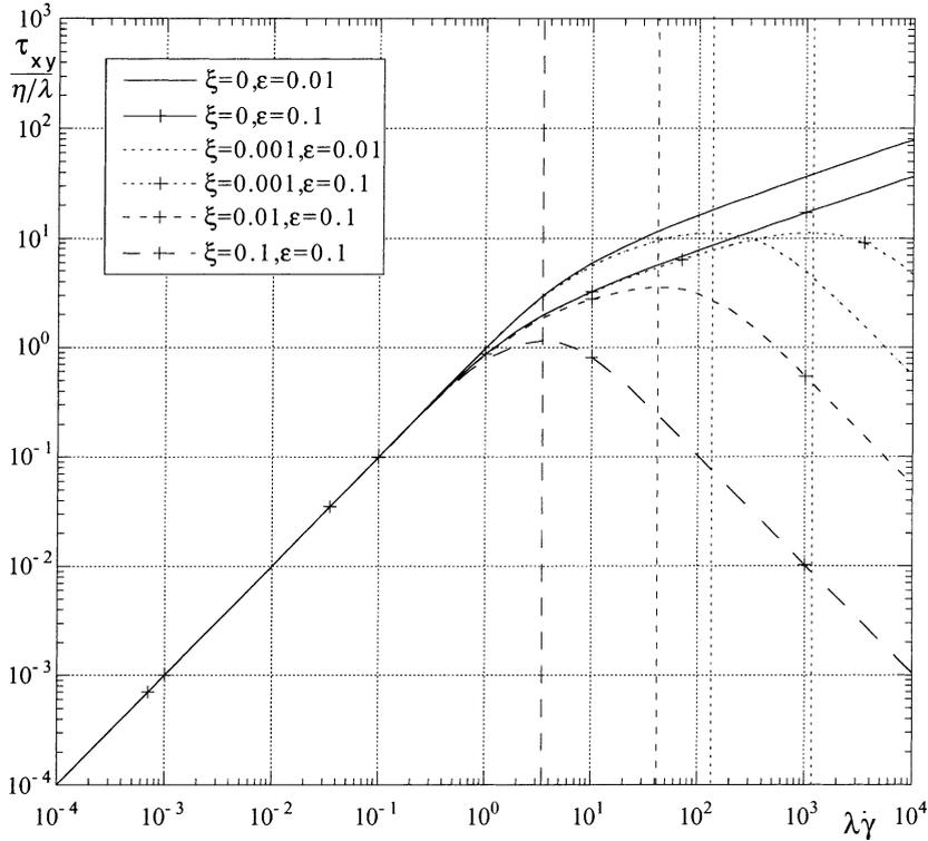
Fig. 1. Variation of the shear stress with shear rate in steady Couette flow for a PTT fluid with linear stress coefficient. Vertical lines:  $\lambda \dot{\gamma}_c$  of Eq. (19).
