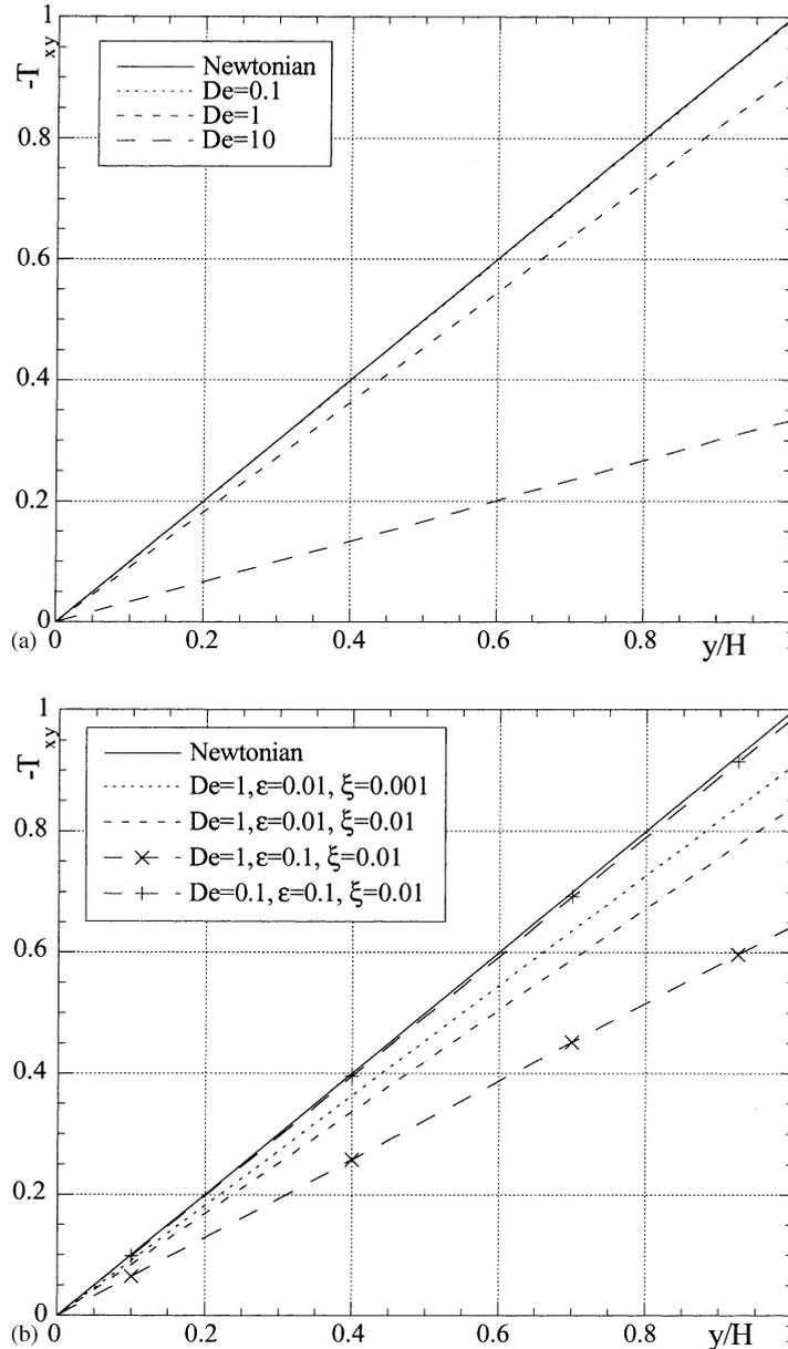
Fig. 7. Transverse profiles of shear stress for channel flow. (a) Effect of Deborah number ( $\epsilon = 0.01$ ,  $\xi = 0.001$ ); (b) effect of  $\epsilon$  and  $\xi$ .
