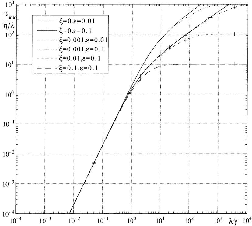
Fig. 2. Variation of the streamwise normal stress with shear rate in steady Couette flow for a PTT fluid with linear stress coefficient.
